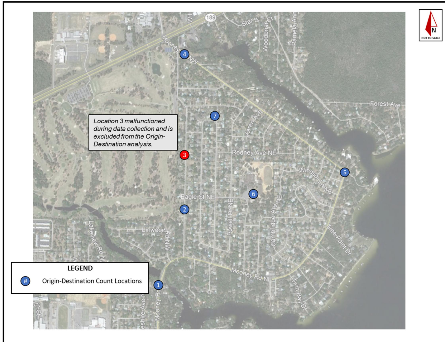
Figure 13: Origin-Destination Bluetooth Sensor Locations
